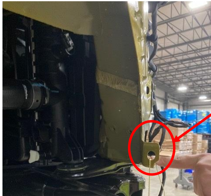
Figure 2 – Passenger Side Preferred Body Hole
