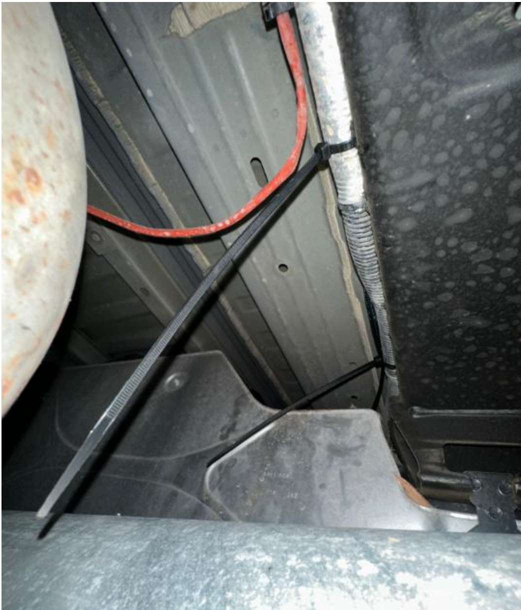
Alternate angle showing the securing of the harness along the cross-member
