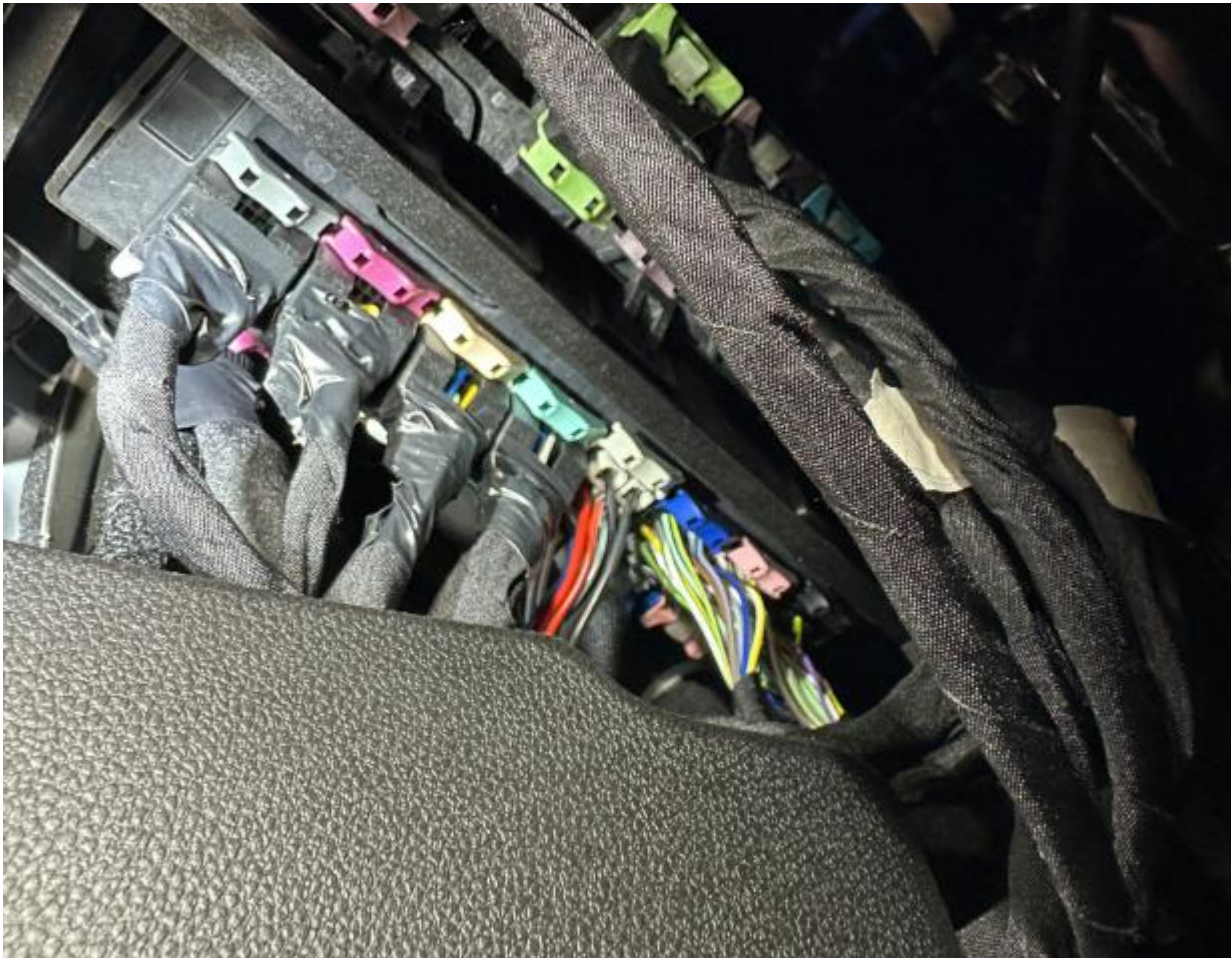
Image showing strain relief fitting on wiring harness (NOT ALL VEHICLES WILL HAVE THESE)
