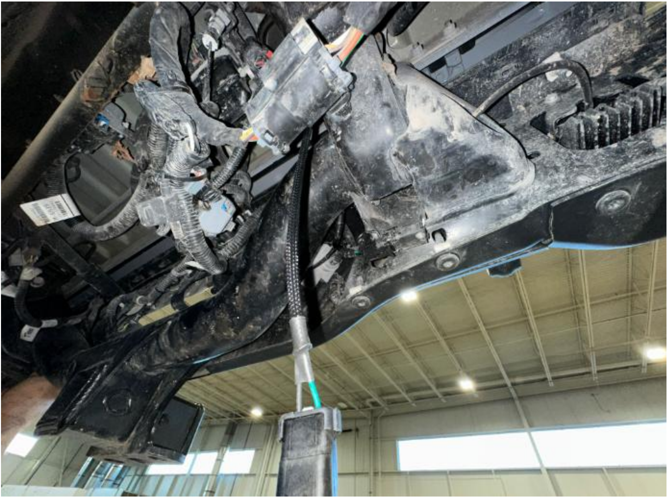
Image showing where the harness end terminates in reference to the trailer hitch.
