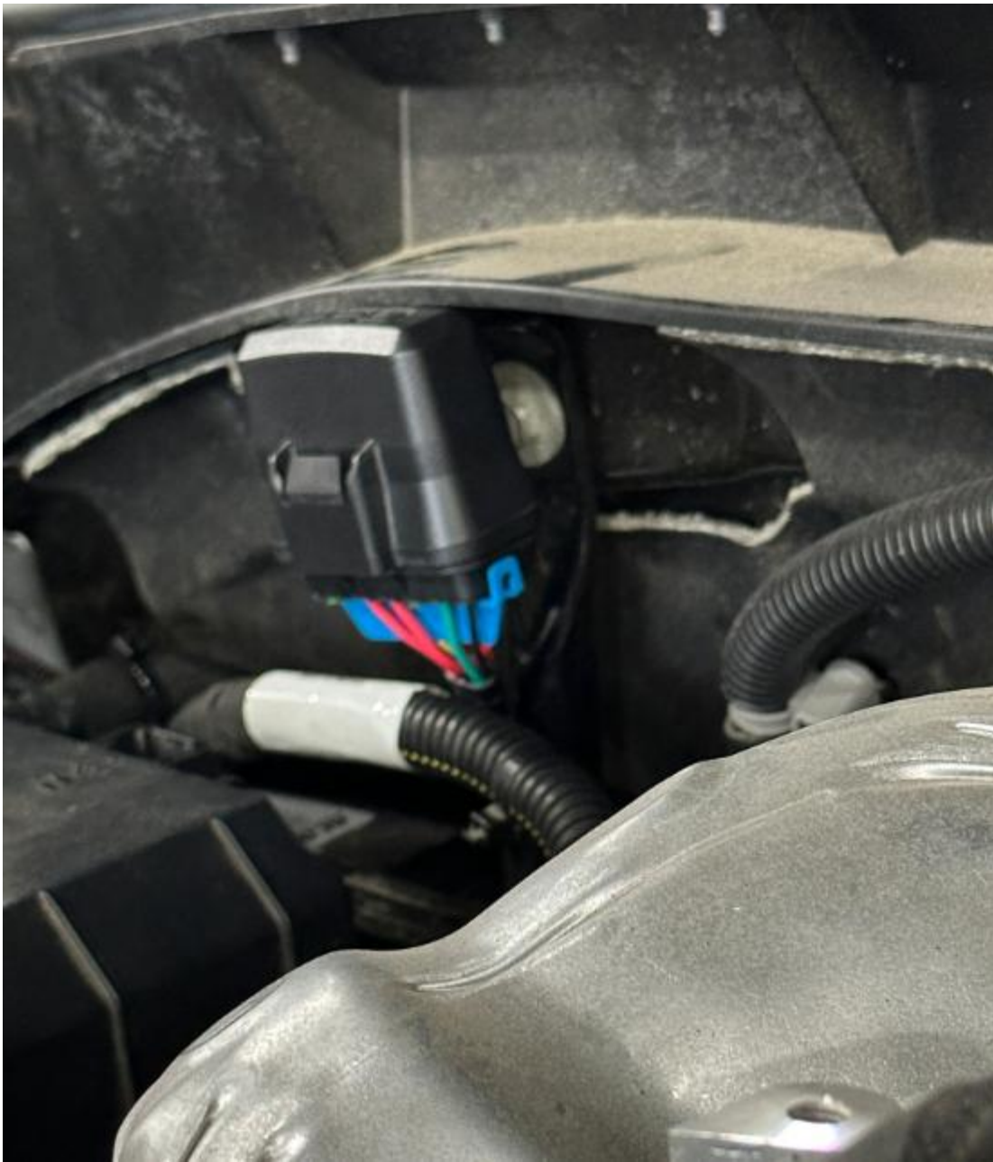
Image showing installation of fuse box between plastic and sheet metal.
