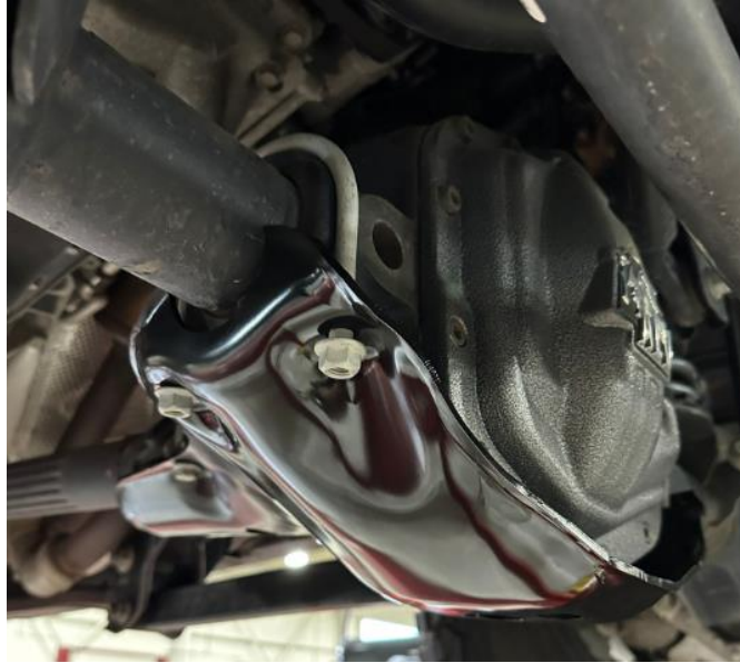
Image 1: Loose install of U-Bolts
