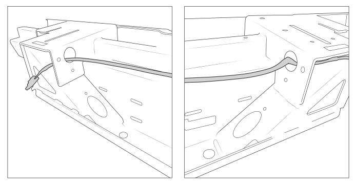
2. Using the provided zipties, mount the harness to the bumper at the provided locations. Simultaneously follow the installation guide of the rear bumper regarding the installation of the vehicle harness. Use the zipties to secure the light harness and factory harness together when applicable.
