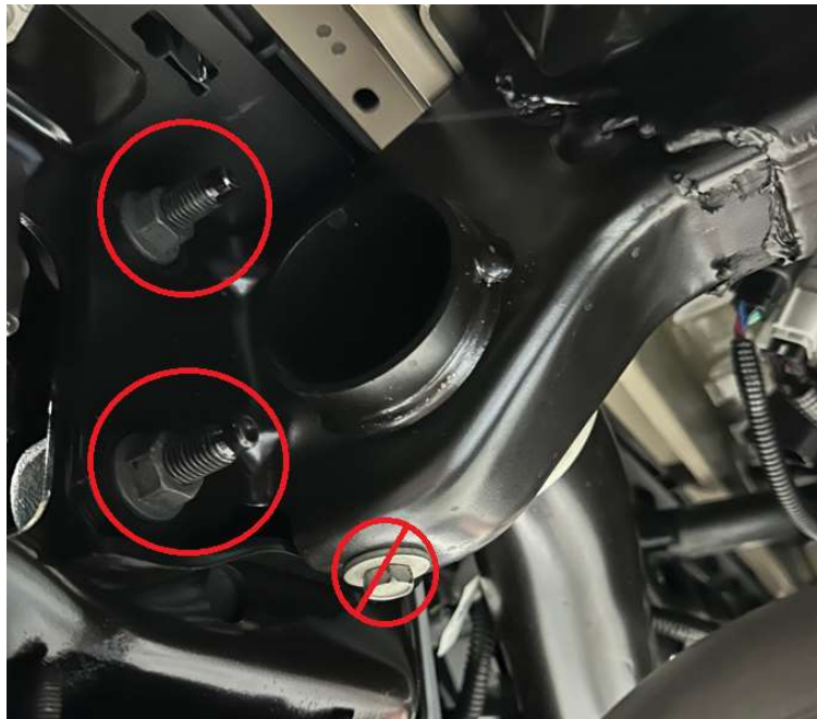
Photo 8: M12 nuts securing bumper
