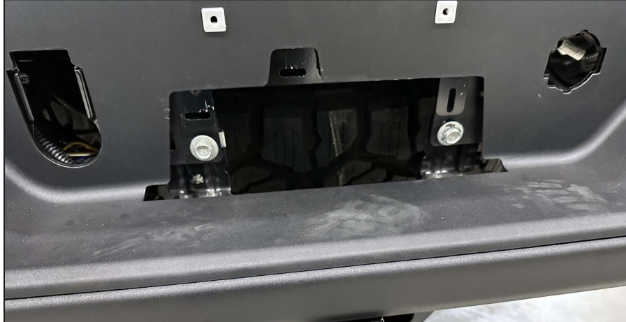
Photo 7: Bolts behind the license plate
