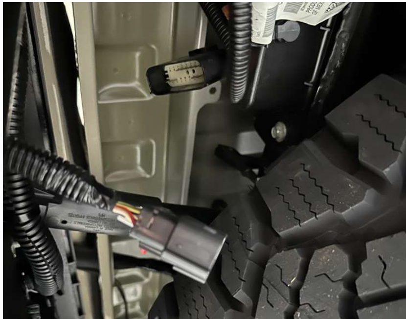
Photo 5: Main wiring harness
