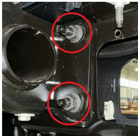
Photo 21: M12 nuts securing bumper
