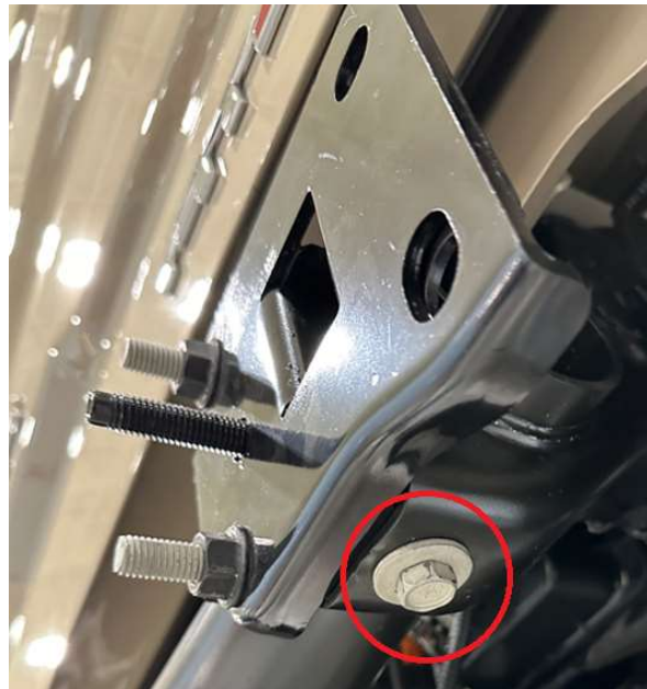
Photo 17: M10 bolt into bottom of hitch bracket
