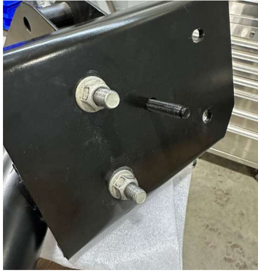
Photo 20: U-bolt bracket secured
