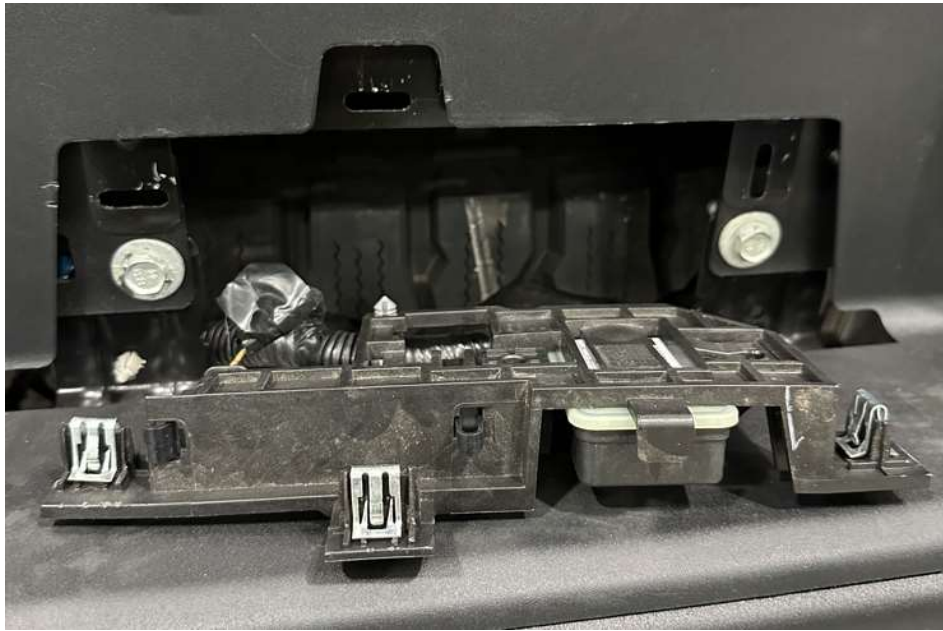
Photo 3: Passive entry sensor removed
