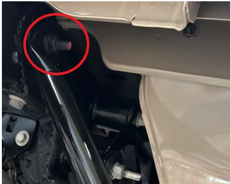
Photo 9: Upper pencil brace mounting location
