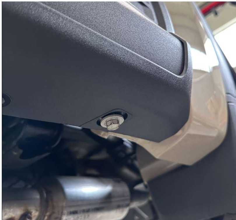
Photo 6: Pencil brace removal
