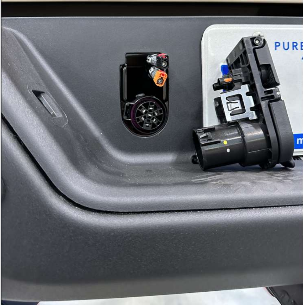
Photo 1: Removal of trailer plug
