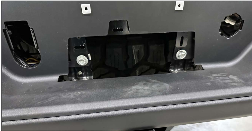
Photo 20: Bolts behind the license plate
