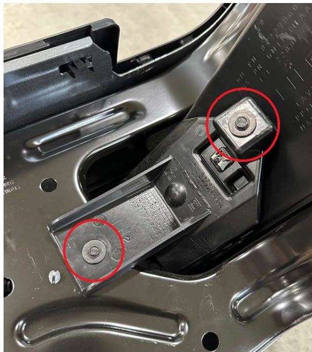
Photo 10: SBZA bracket removal
