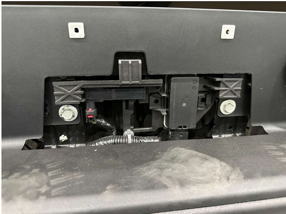
Photo 2: Passive entry sensor behind license plate
