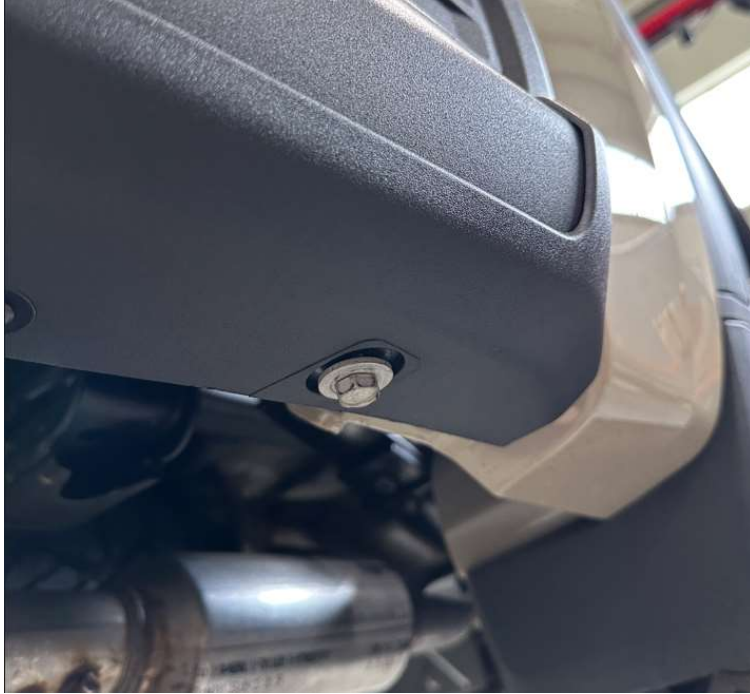
Photo 23: Pencil brace installation
