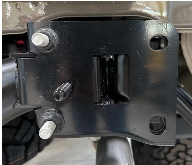
Photo 16: Hitch bracket installation
