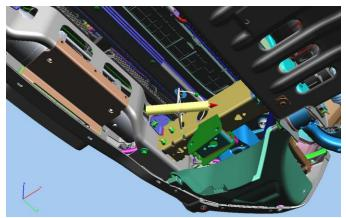
6. Route the Blue, White, and Yellow marked harness end terminals through the passenger side bumper window. Secure each of the terminals to the corresponding color winch threaded studs by holding the lower nut on the stub and fastening the upper nut clockwise to a torque of 14 Nm. Include a lock washer on each threaded stud per the diagram shown here.
