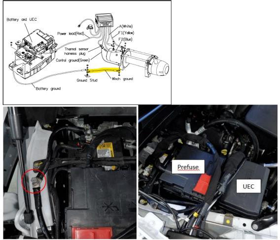
8. At the winch route the chassis ground stud to the winch ground cable below the bottom of the bumper and place the end terminal on the winch's bottom threaded stud. Also, place the control ground (green with outer white sheathing) wire connector on the same winch bottom threaded stud. Secure both terminals to the same winch threaded stud by holding the lower nut on the stud and fastening the outer nut clockwise to a torque of 14 Nm. Include a lock washer on the threaded stud.
