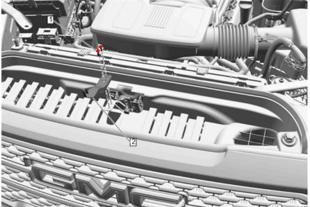
10. To complete the winch controller on/off switch installation attach the quick connect male end from the button switch to the female end quick connector from the winch controller.
