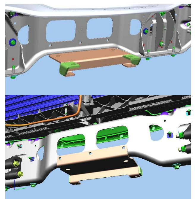
4. Insert square nuts from the winch kit box at 4 places in the winch mounting feet pockets.\_\_\_\_\_
