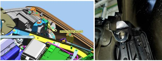
5. Loosely drape the larger primary winch controller mount bracket over the passenger side frame rail behind the front head light and outside the battery and in front of the hood hinge. The bracket's top rear bolt hole will align with the double ended stud.
