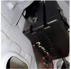
11. At the front middle controller edge install a M6 -1.0 x 12mm bolt through the back of the large primary bracket into the small secondary bracket (item <sup>(1)</sup>) in the bracket and fastener diagram above). The bolt head will be next to the frame rail and the bolt threads will point outward. Fully tighten the flange nut (item <sup>(3)</sup>) in bracket and fastener diagram above).
