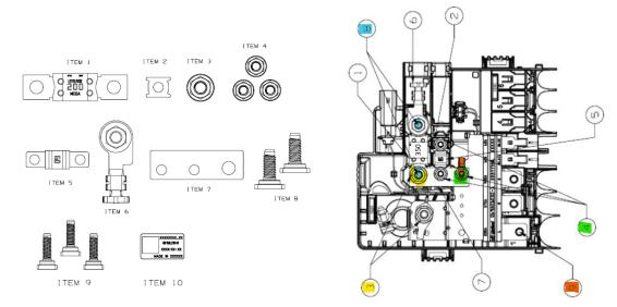
350A Mega Fuse – Note: Discard the 200A Mega Fuse contained in Block Kit 84669070
