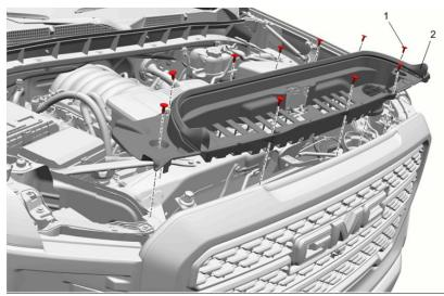
9. Reinstall the secondary release latch (2) and hood latch actuator bolt (1).
