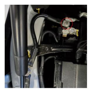
2. Attach the wired remote cable to the wired remote plug at the winch controller.
