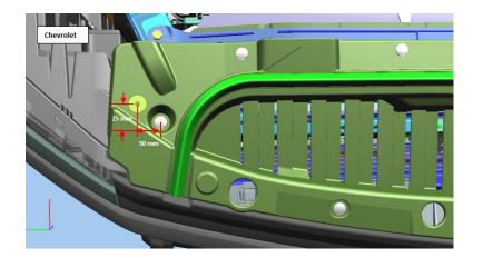
3. Drill a 5/8-inch diameter hole for the on/off switch.
