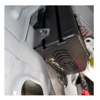
13. For the large primary bracket's lower attachment hole install the M8 x 1.25 x 20 hex head bolt with conical washer in the vehicle frame rail (item 11 in the bracket and fastener diagram above). Use a magnetic extension pickup tool to feed the bolt through the large oval shaped window in the frame rail down to the circular bolt hole opening.
