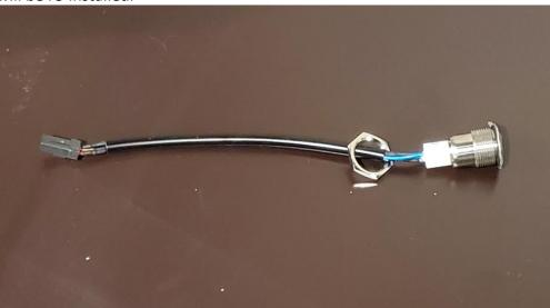
5. Thread the included washer (24 mm OD, 16 mm ID) over the quick connect male end of the on/off switch until it is seats under the switch button rim.
