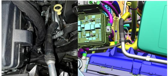
3. Route winch harness bundle down from the UEC to the frame front passenger corner through the chassis wiring channel.
