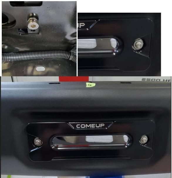
3. Position the winch mount platform aligning the three attachment bolt holes behind the three bumper cross member bolt holes. Install three M10 x 1.5 x 25 flange bolts in the holes with the bolt head on the front side of the bumper cross member. Secure three M10 x 1.5 hex flange nuts on the back side of the bumper. Torque to 58 Nm.
