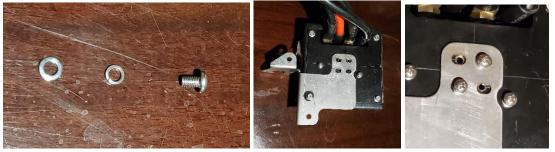
7. Place the wired remote plug in the secondary bracket receiving hole. Securely tighten the two wired remote plug mounting bolts and nuts into the bracket.
