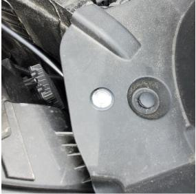
7. Reinstall the thin 2.5 mm thick hex nut by threading it over the quick connector. Screw the hex nut to the threaded switch button housing until its flush with the underside of the air intake splash shield. Firmly tighten the hex nut.
