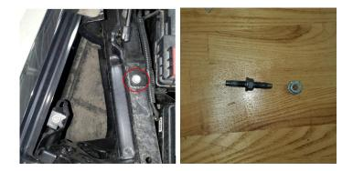
4. For GMC trucks <u>only</u>, bend the upper fender bracket tab located behind the passenger head light (see pictures below) down 90 degrees to provide extra clearance for the winch control module. Use a channellock or vise grip pliers. This will provide added clearance during the installation process.
