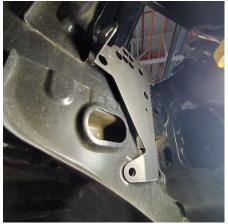
6. Attach the small secondary bracket to the control module with the two M5 x 8 mm screws, flat washers and lock washers as shown. These fasteners will be in the winch kit with the controller and harness.
