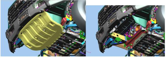
3. Remove the M8 bolt that secures the front battery tray support to the inner frame rail. Replace it with the double ended M8 stud.
