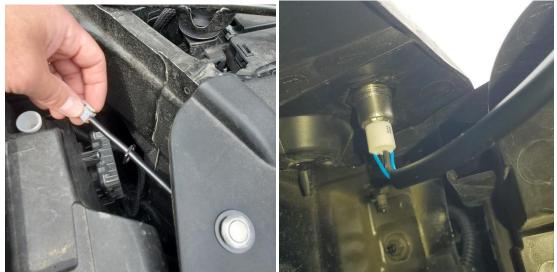
8. Reinstall the air intake splash shield (2) at the top of the grill with intake air baffle retainers (1).
