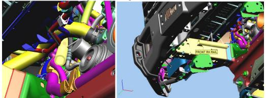
5. Continue routing the winch wire harness forward along the front passenger side frame rail to the passenger side of the winch.
