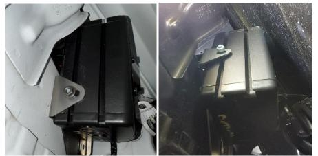
10. At the lower front controller edge install a M6 -1.0 x 12mm bolt (item <sup>(1)</sup>) in the bracket and fastener diagram above) through the back of the large primary bracket into the small secondary bracket. The bolt head will be next to the frame rail and the bolt threads will point outward. Loosely tighten the flange nut a few turns (item <sup>(3)</sup>) in bracket and fastener diagram above).
