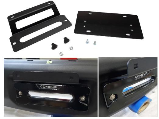
b. Fairlead: From the winch kit box locate the fairlead and two M10 low profile bolts with washers and nuts. Place the fairlead on the front side of the bumper. Place the bolt head with lock washer on the rear inboard side of the bumper in two places and press the bolt through the fairlead on the front side. On the forward side add a flat washer and nut in two places. Torque the nuts to 58 Nm each.
