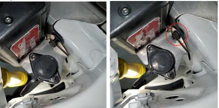
12. Fully tighten T-slot nut and lower front controller edge flange nuts.
