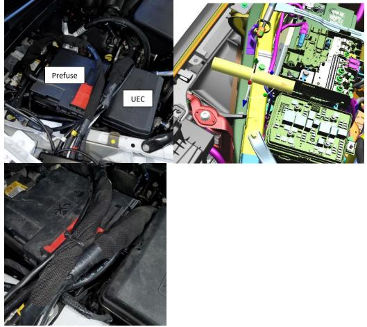
2. Route winch harness bundle downward between the inboard side of the UEC and outboard side of the hose heater outlet assembly.
