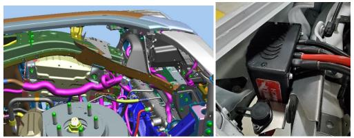
9. Loose fit the M6 -1.0 x 16mm bolt head (bolt ④ in bracket and fastener diagram below) into the control module T-slot closest to the controller's flat side next to the frame rail. Guide the bolt threads through the bracket slot manipulating the bracket rearward to insert the bolt. Loosely attach the flange nut on the bolt a few turns (nut ③ in bracket and fastener diagram below).
