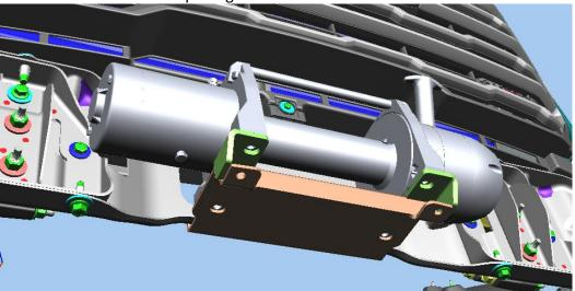
6. Bolt the winch to the front bumper mounting platform at the four mounting feet into the square nuts with four M10 flange hex head bolts from the winch kit box. Torque the four bolts to 58 Nm. The front two bolts will require a crow's foot extension on the torque wrench to access the bolt head and achieve the 58 Nm torque (see pictures below). Use the crow's foot at a 90-degree angle to the torque wrench to maintain the moment arm and achieve the 58 Nm torque.
