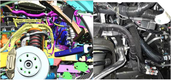
4. At the bottom of the chassis wiring harness channel route the winch wiring harness inboard and forward along the front right hand frame rail
