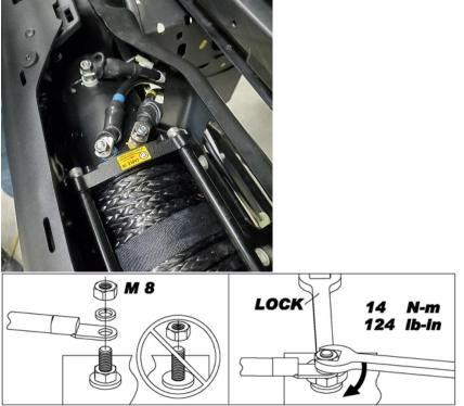
7. Install the separate longer black 2AWG cable from the chassis ground stud to the winch ground. Attach one end to the chassis ground stud located at the rear passenger underhood corner. Route the other end on the same path as the winch controller to winch harness between the Prefuse and UEC. Route the chassis ground stud to the winch ground cable down through the chassis wiring channel, and then downward and forward to the winch.
