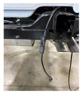
2. Pull the plug from the previous step into the vehicle, running under the two vehicle harnesses and along the frame. Run the cord behind the shock mount.
