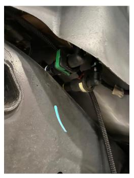
4. Next feed the wire harness above the next vehicle harness that comes after the fuel lines.
