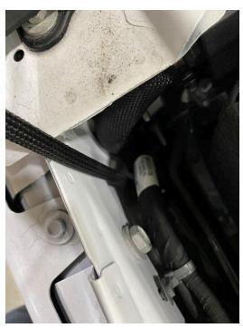
7. Finally connect the corresponding wires to the vehicle aux wires according to color.
