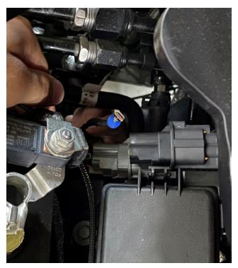
4. When attaching the rear bumper, connect the end of the harness with the harness that resides in the AEV rear bumper.
