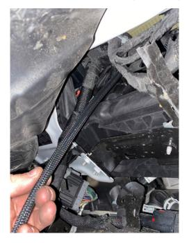
3. Feed the wire underneath the two wire harnesses shown.
