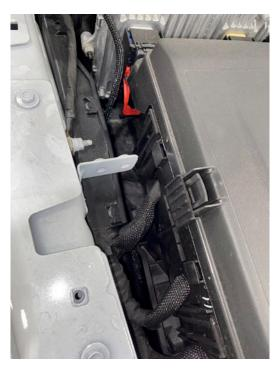
4. Then feed the wire between the body of the vehicle and battery block as shown.
