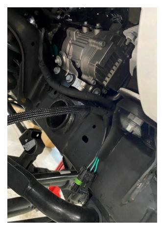
2. Access the cavity behind the wheel liner and run the wire up to the top of the vehicle.
