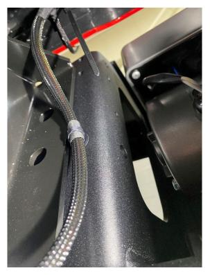
3. Ground the harness to this position near the battery and continue to run the wire around the back of the battery in order to connect it to the Ram aux plug.
