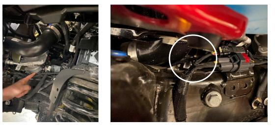
2. When adding the bumper to the vehicle use the christmas tree clip to feed into the lowest hole in the bumper assembly.
