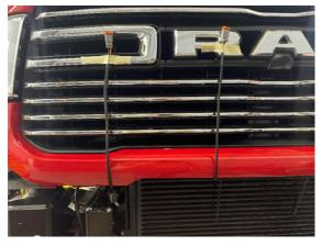
3. When adding the bumper to the vehicle use the christmas tree clip to feed into the lowest hole in the bumper assembly.
