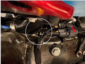
2. Use the provided edge clip ties to mount the harness to the frame.
