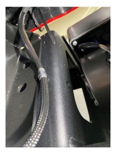
4. Ground the harness to this position near the battery and continue to run the wire around the back of the battery in order to connect it to the Ram aux plug.
