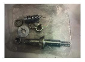
Included with the hardware for the rear suspension is a bag with two thick washers and two thinner washers, the thicker ones are used to space the front transfer case crossmember down for driveshaft clearance, the thinner ones are used on the rear swaybar end links.
