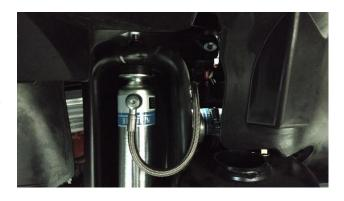
Rear: Reservoir should be clamped to the shock body, ensuring that the main shock body banjo fitting is facing away from the frame and the hose is routed as shown in the photo to prevent pinching or interference during articulation. For reference, this is on the right side of the vehicle.
