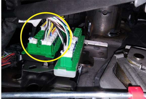
3. Install the AEV Programming Harness into any open slot in the green Star connector.
