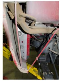
Figure 2 Remove plastic support and metal support rods
