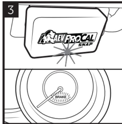
3 Wait for a blinking GREEN light on the SNAP and a blinking BRAKE light on the speedometer.
