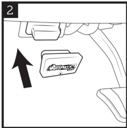
Insert ProCal SNAP into the OBDII port.
