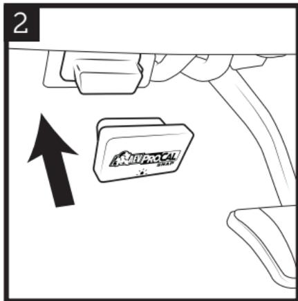
2 Insert ProCal SNAP into the OBDII port.
