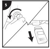
Turn the key to the "off" position then remove the ProCal from the OBD port.
