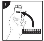
Set the DIP switches on the back of the ProCal using this Quick Reference Guide for the function you wish to program.
