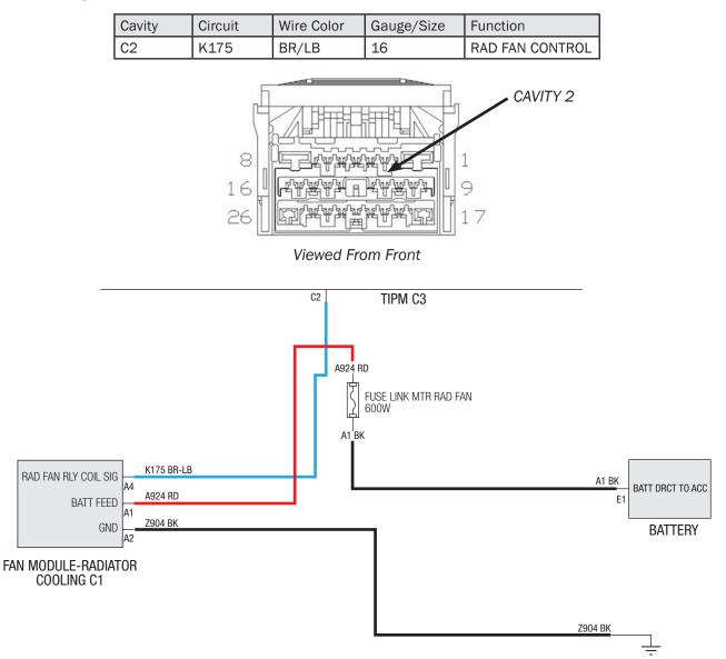
3. Use the ProCal to change the fan setting in the TIPM. Turn the ignition key to the RUN position, apply the ProCal settings shown then plug the ProCal into the OBDII port. Wait for 2 horn honks then remove the ProCal and turn ignition to OFF. Programming is complete.
