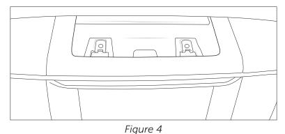
6. Clip the radio bezel back in at this point and reinstall the screw above the 115V outlet (if equipped).
