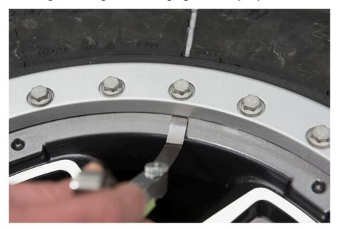
9. Inflate tire to seat inner bead. Do not exceed 45 PSI to seat bead.
