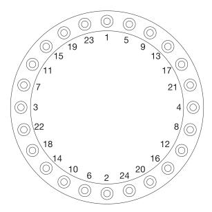
NOTE: TO PREVENT RING DAMAGE IT IS VERY IMPORTANT TO FOLLOW THIS TORQUE SEQUENCE, MAKING SURE TO MAINTAIN A UNIFORM GAP BETWEEN THE RING AND THE WHEEL DURING THIS PROCESS. THIS PROCESS IS TIME CONSUMING BUT DO NOT SHORT CUT OR USE POWER TOOLS.
