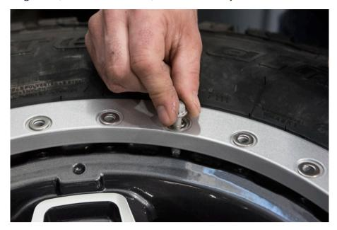
4. Tighten bolts using the torque sequence provided to uniformly draw the ring down on the tire bead. Torque all bolts to 10 lb-ft.
