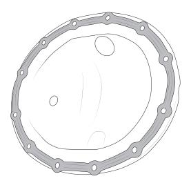
7. Place the new differential cover and factory gasket in the correct orientation and install all 11 socket head cap screws and one flat head screw finger tight and then tighten in a criss-cross fashion to 25 lb-ft.
