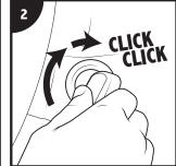
Insert the key into the ignition \* and turn TWO clicks to put the vehicle in the "run" position.
