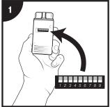
Set **all nine** DIP switches on the back of the ProCal using this Quick Reference Guide for the function you wish to program.
