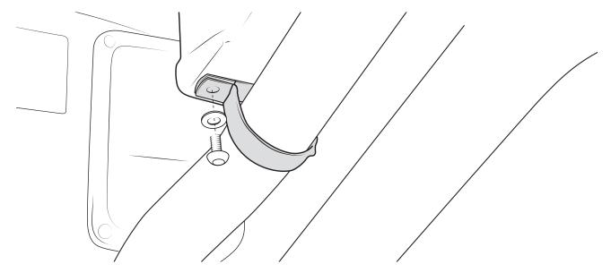
5. Mount tire to Tire Carrier securing lug nuts. Tighten the tire mount bolt on the back of the Tire Carrier until the tire is pulled tight to the Fuel Caddy. Use a hammer and a flat head screwdriver to bend the tongues of the safety washer against the head of the bolt.
