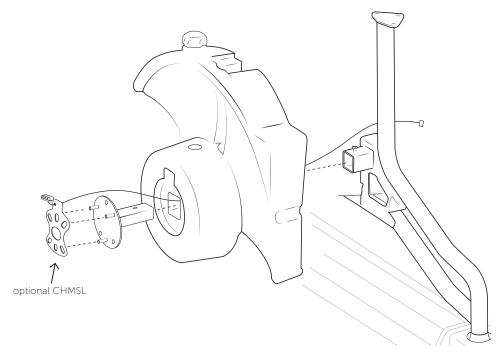
2. Lift Assembly onto the Tire Carrier. Position back plate bracket behind Tire Carrier as shown and secure Fuel Caddy with three 5/16"-18x Button Head Bolts and 5/16" washers. Thread the Tire Mount Bolt with saftey lock washer through the back of the Tire Carrier to secure.
