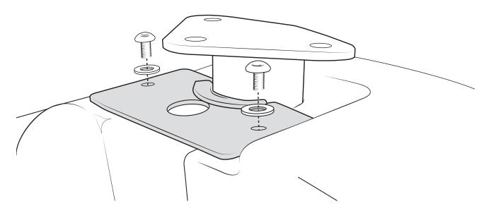
4. Position "P" clamp around Tire Carrier tube as shown and secure using one 5/16"-18 Button Head Bolt and 5/16" washer.
