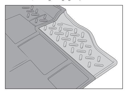
You may also want to trim out the two small circles at the front end of the Cargo Liner to retain access to the tie down points in the floor of the Jeep.
