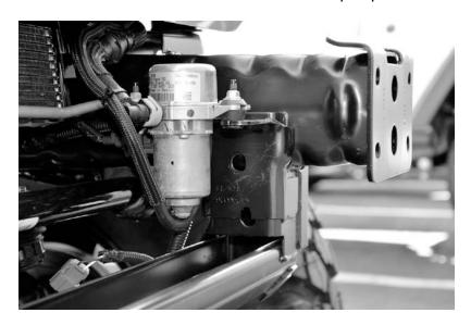
2. Assemble the supplied AEV vacuum pump bracket to the winch mount as shown using the supplied hardware.
