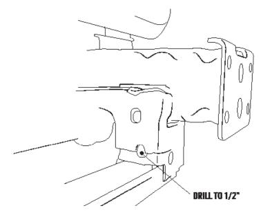
4. Depending on the winch being installed, you may need to trim the factory vacuum pump bracket for necessary clearance (as shown). The photograph on the next page shows a marked-up bracket showing the area that needs to be trimmed.
