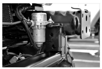
2. Assemble the supplied AEV vacuum pump bracket to the winch mount using the supplied hardware (as shown).
