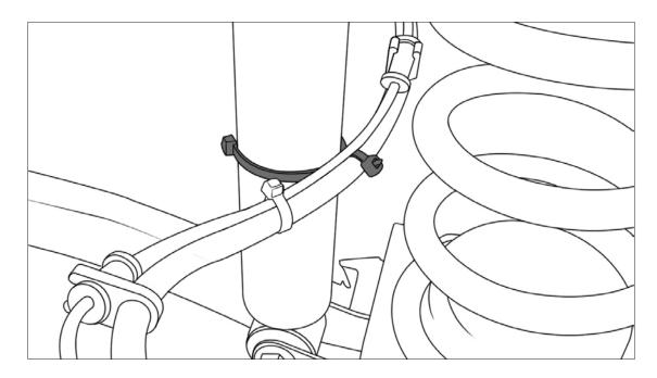
For 2011 and newer models, use supplied zip ties to secure the brake line to the shock as shown.
