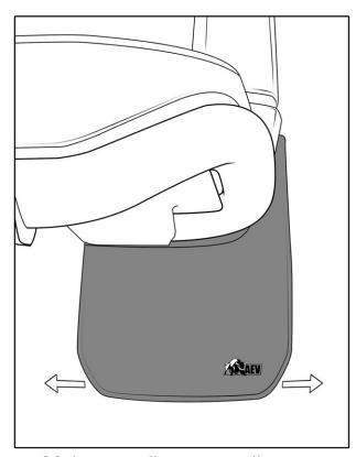
4. Make any alignment adjustments before final tightening.
